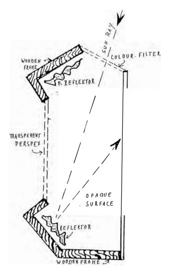
Diagram of the vertical cross section of the Robot Projector for 'Light Symphony, No. 1'.
