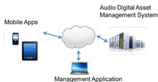
Fig 3. Overall software architecture, 2015, all rights: Gauss Institute Bitola
