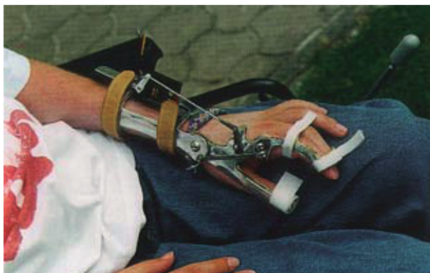
the orthosis (mechanical hand) of the paralysed patient is being steered by the power of his own brain.
