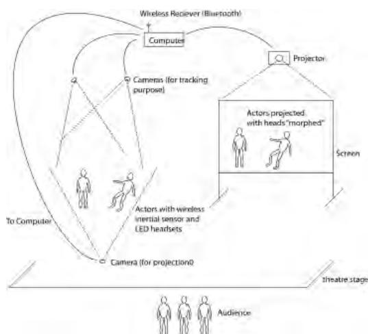
Figure 2: Setup of augmented reality system for theatre. The audience sees the juxtaposition of real and augmented spaces.
