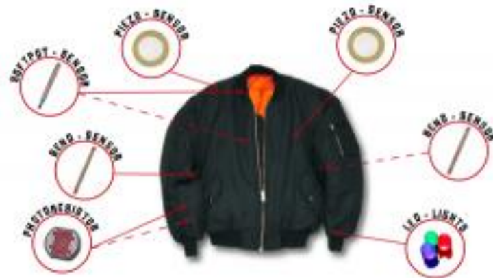
Sensor layout for the first prototype VJacket, 2010. It includes a LED on one wrist and light sensor on the other so you can cross wrists to trigger video effects. Image copyright A. Zingerle.
