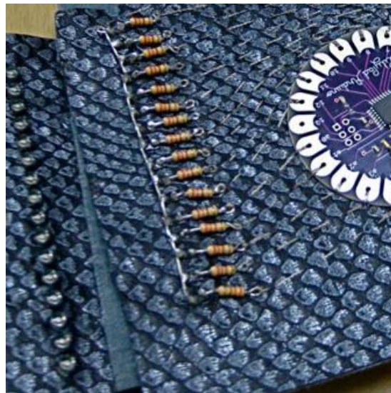
Fig 2. Body Graffiti(Testing Prototype, hand sewn electronic circuit with LilyPad Arduino), 2009, Younghui Kim
