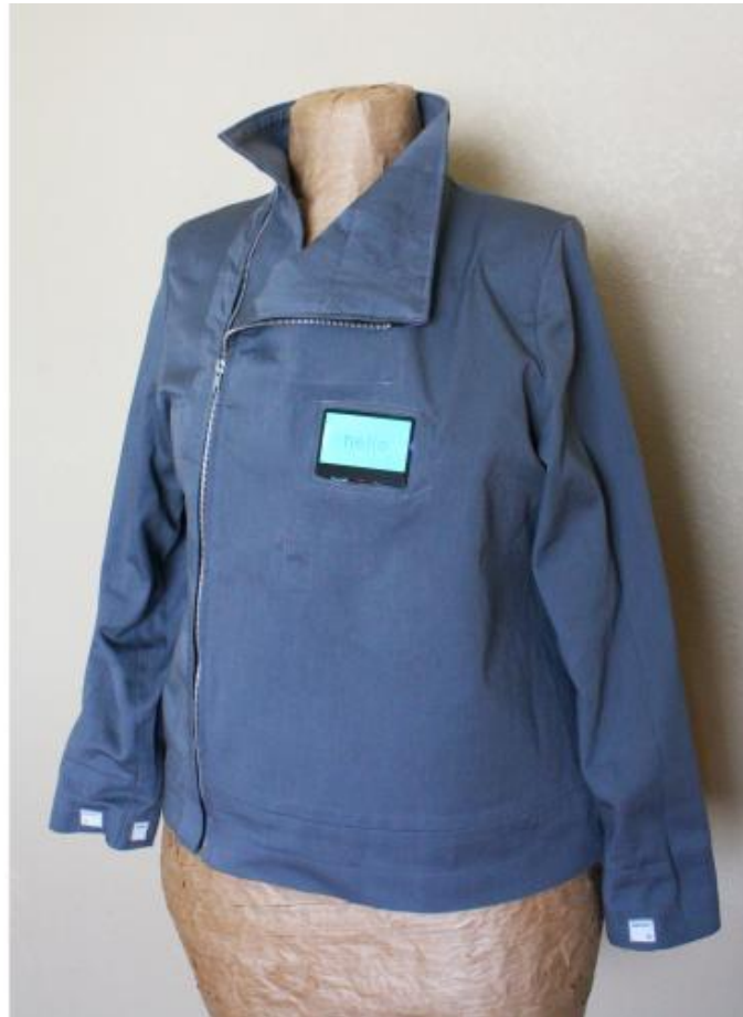
Kristin Stransky Mallinger, intraInter socialite, 2011, Emoticon jacket with LCD screen, Lilypad Arduino board and force sensors (artwork and photography © 2011 Kristin Stransky Mallinger).
