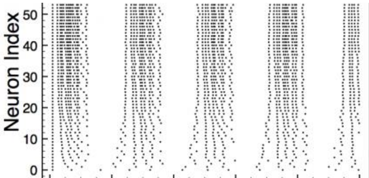
A raster plot showing the spiking behaviour of simulation of a network of 64 neurons modelled using the Izhikevich Model (2004) copyright Kevin McCracken.
