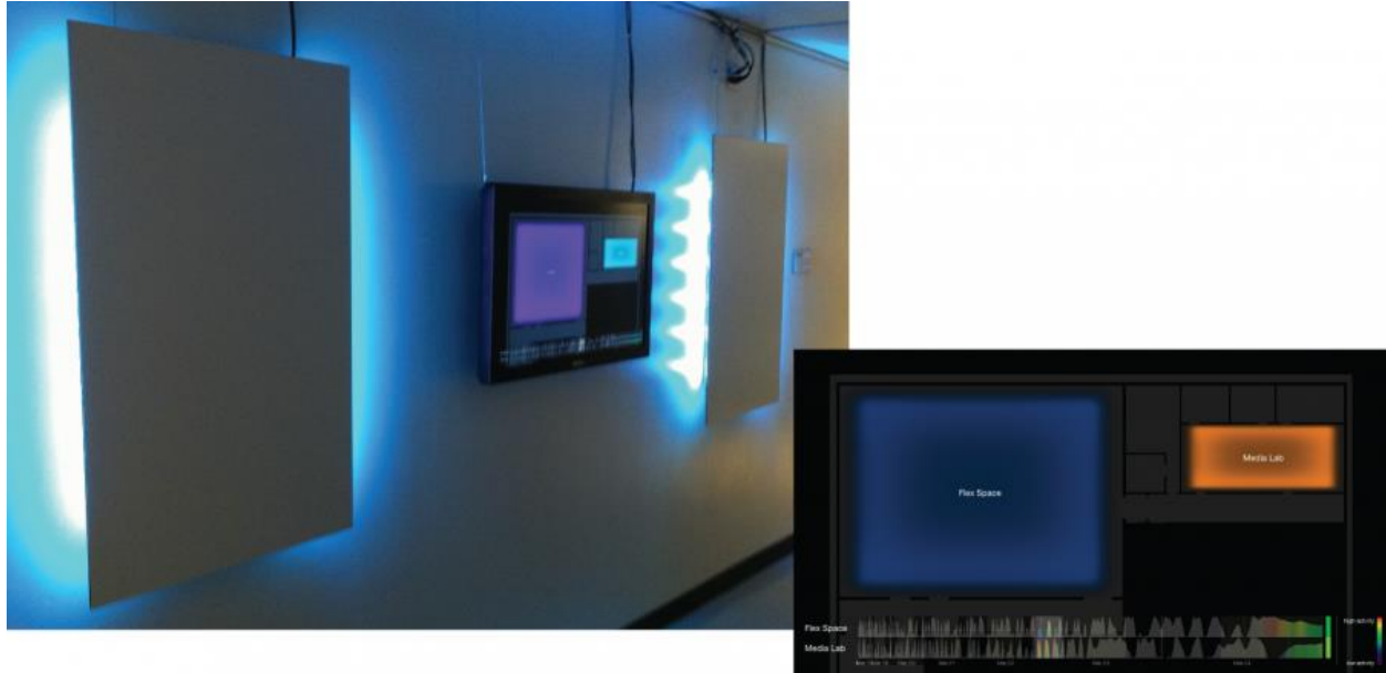
Fig 2. Building with a Memory uses wall-mounted LED lights and a video display (see inset detail) to present current and historical human physical activity in a multi-use workplace. Copyright Arizona State University 2011.
