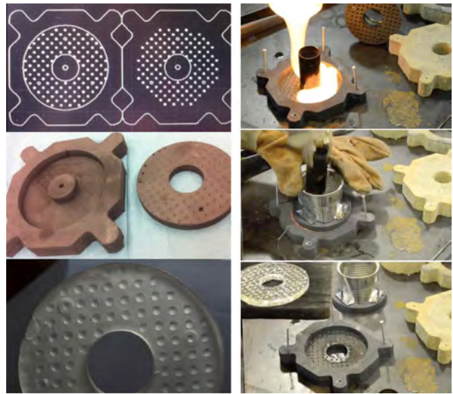
Fig. 8. Reinterpreting the making of ancient Chinese bi disks, © 2013, Hursty. Top left, CAD drafting, Middle left, waterjet cut graphite mold, bottom left, finished glass bi with press formed hole. Right column shows bi pressed from molten glass.
