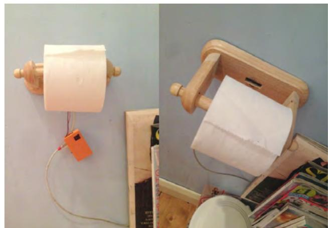
Fig. 1. First working prototype of the instrumented toilet roll holder. © Chris Speed.
