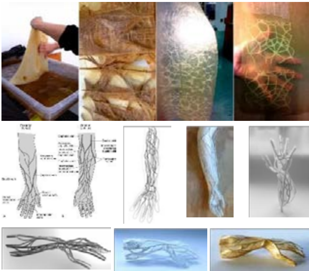
Figure 2: Stages of the fabrication process, bacterial cellulose growth and harvest; drawings, 3D doodle prototypes, 3D PLA plastic print, and a photograph of the bacterial cellulose clad prototype.
