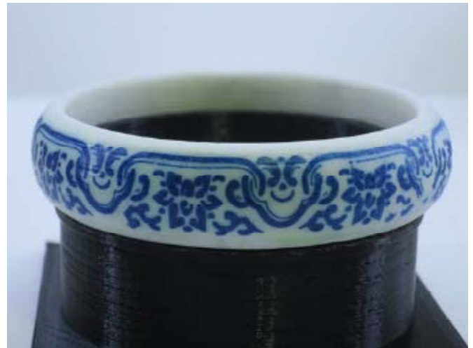
Fig.5 Vector graphic printed on FDM printed PLA bracelet © copyright Authors, Photo Authors
