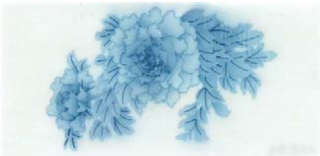
Fig.3 Gradient and line graphic printed on flat ABS plate © copyright Authors, Photo Authors
