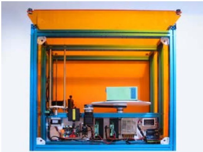
Fig. 1 Custom CNC controlled laser positioning machine for laser exposure experiments © copyright Authors, Photo Authors
