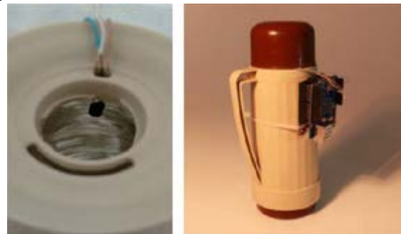
Fig. 1 –sensor LM35 sensor embedded inside the container of the
