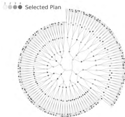
Figure 1. EPOS agents performing collective decision making over a self-organized tree topology for the optimization of the aggregate energy demand. Agent locally generate four energy demand plans and cooperatively make a selection
