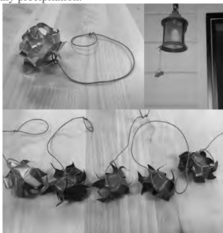
Figure 1. left: An example of the cut and folded copper foil before being placed outdoors; center: example location of where the pieces were located outside; right: The copper pieces after being placed outside for several months.
