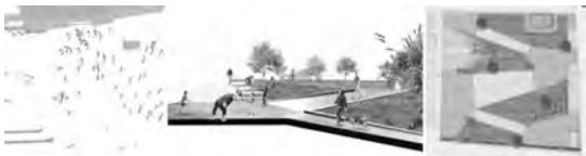
Figure 4. This series of images shows how foot traffic was studied at an urban scale. These simulations impacted the design of the park as flow was used to help articulate ramps and terraces.
