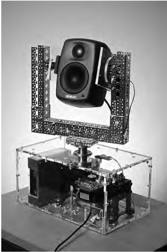
Figure 1. The speaker.motion mechatronic loudspeaker
