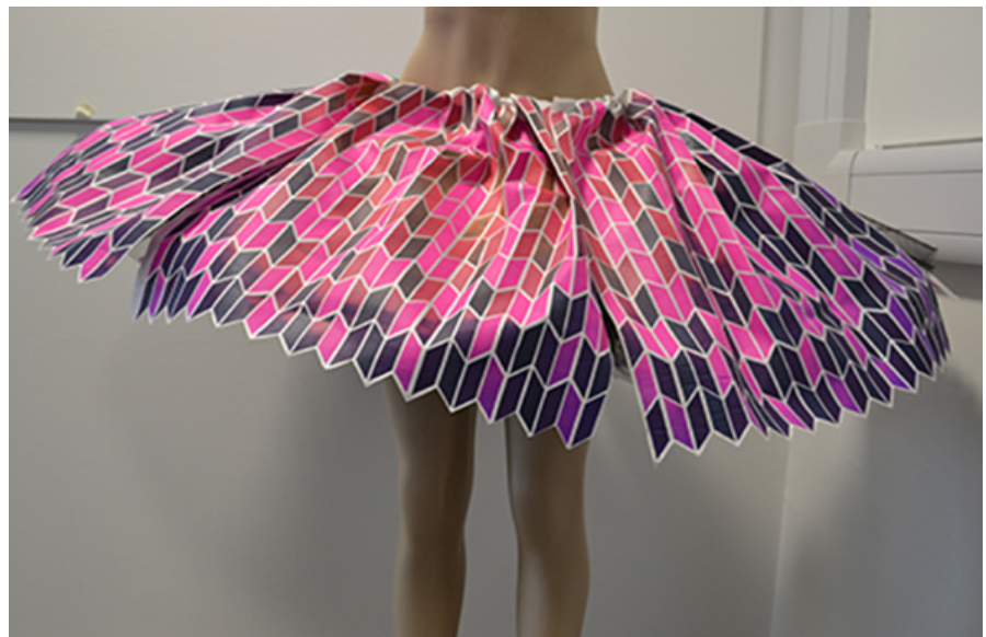
Fig. 7. Thermochromic and fluorescent screen printed tutu in mid change (Photo © Lynsey Calder)
