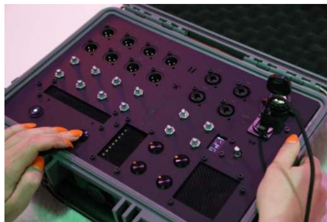
Figure 7. Prototype of a multichannel interface for atmospheric soundscape immersion.
