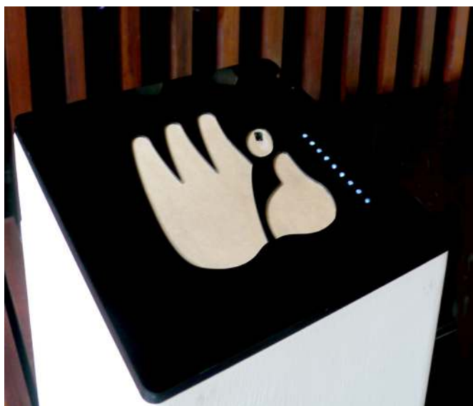
Figure 6: Heartbeat sensor and Led light of 1~10 level
