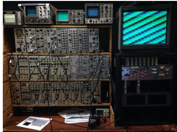
Figure 2. Dan Sandin’s IP (1971–73). Note that the cables act as “patches” between the modular analog computers that process the video signal. Photo by Rosa Menkman, taken April 3, 2015, at the School of the Art Institute of Chicago, where the IP operates to this day. ©Wikipedia.
